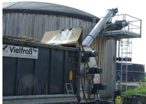
Feeder, first fermenter and (far right) storage tank. Photos: F. Gerlach, FiBL
